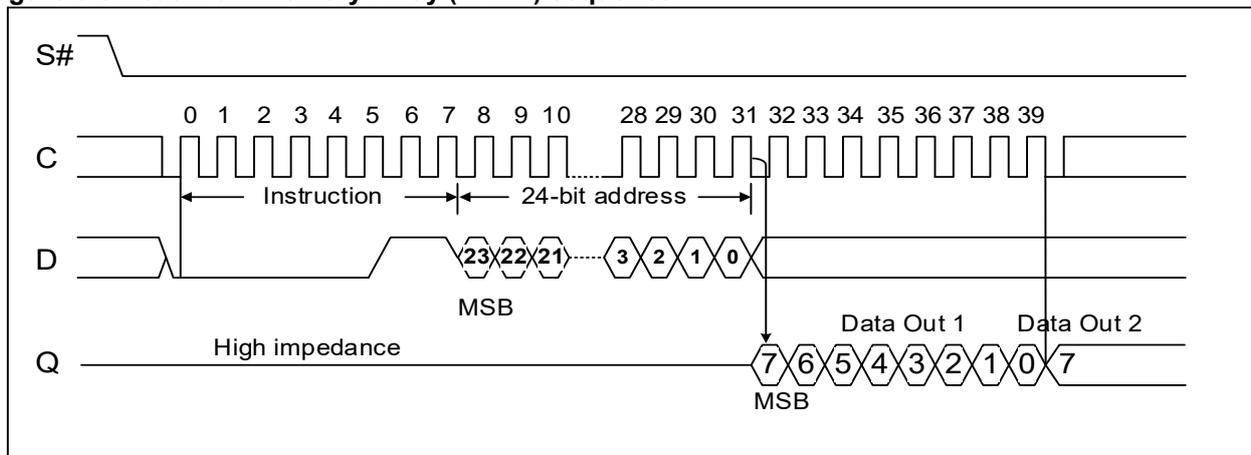
The instruction is not accepted, and is not executed, if a Write cycle is currently in progress.
