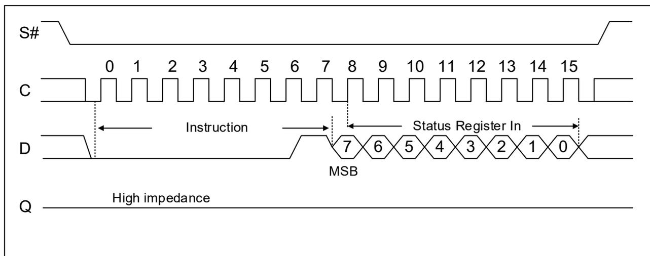
Driving the Chip Select (S#) signal high at a byte boundary of the input data triggers the self-timed Write cycle that takes  $t_W$  to complete (as specified in AC tables in: DC and AC parameters).
